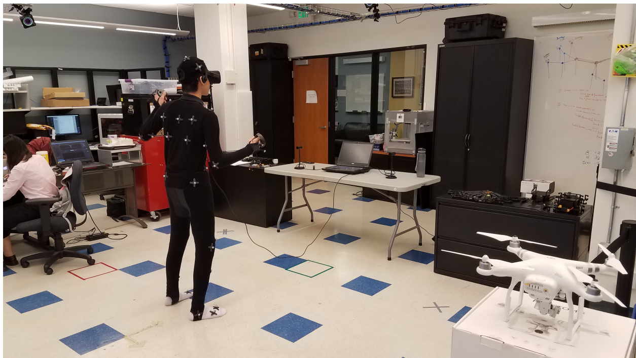
Figure 3.2: Our data capture setup. One laptop (middle) runs and records VR inputs, while a second (left) operates the motion capture system.
