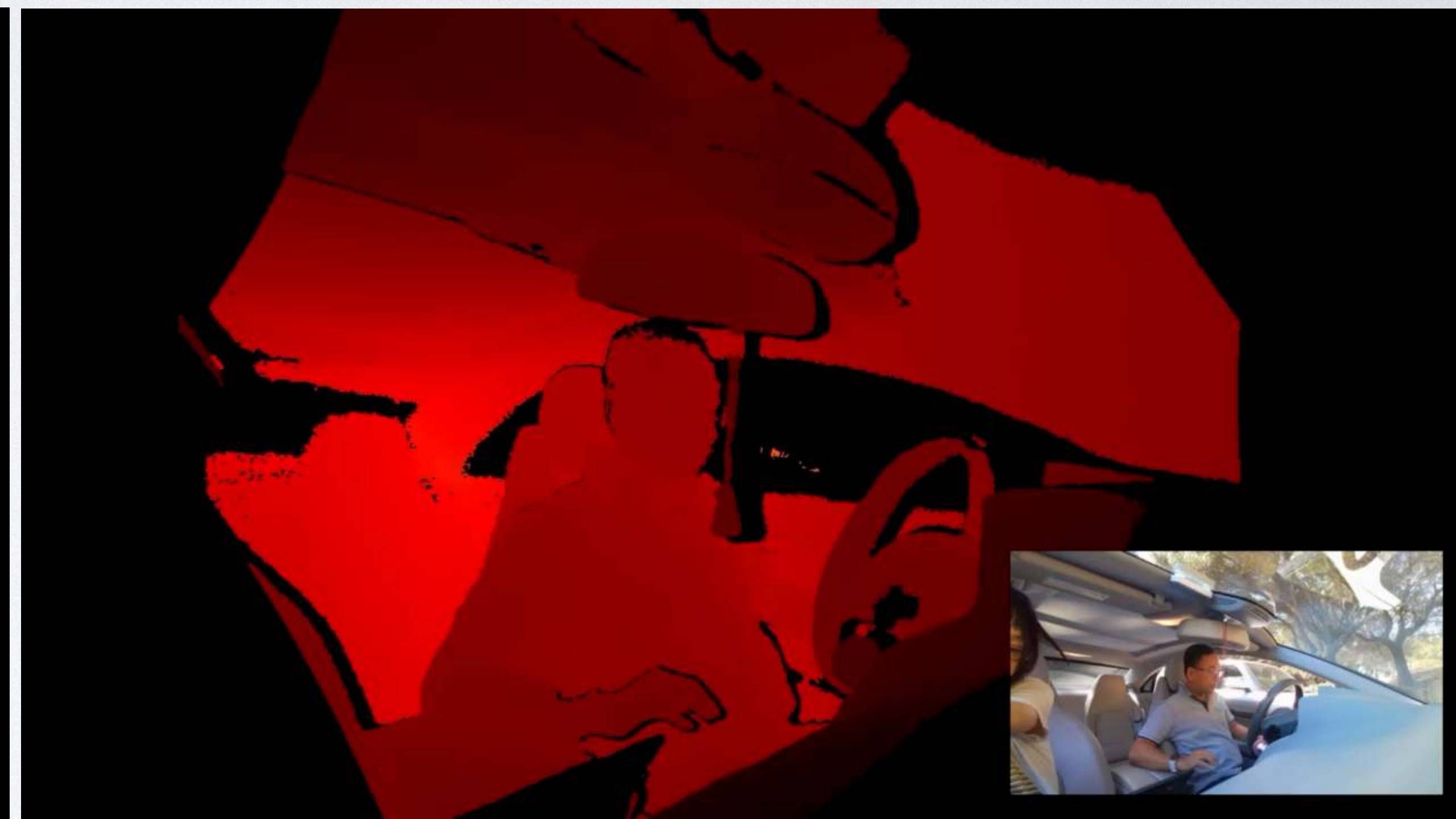
Azure Kinect, Time-of-Flight technology
