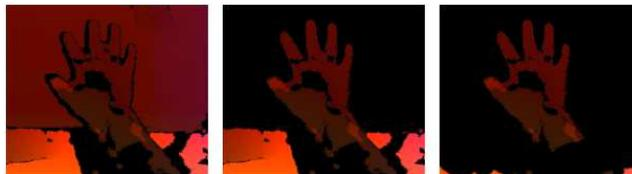
Figure 2: Pipeline to extract the hand cluster from background noise. We first remove all planar surfaces which the hand might contact with. Next, we remove all background noise and clutter.
