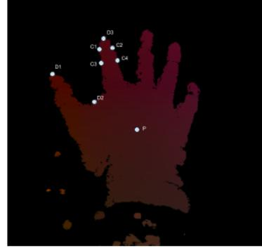
Figure 5: Keypoints used for finger classification. D1, D2, and D3 are computed from defects in the convex hull. P is the center of the palm. C1, C2, C3, and C4 are nearby points to the defect start and end.
